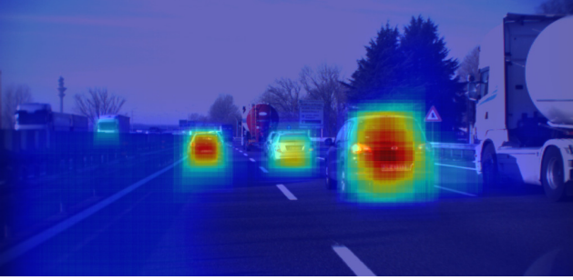
Figure 3: WaldBoost attention heatmap. For each pixel in the images we visualize the number of weak classifiers that was evaluated. For blue regions the subwindows were rejected almost immediately, while for red regions the entire cascade was evaluated. 1
